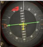
Horizontal Situation Indicator. With glideslope support and heading bug. Connected to NAV1.
