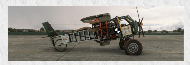
Also: The wings are relatively lightweight (fuel tank is located where the passenger seat would be in a normal aircraft). The weight is then not only centered on the roll axis, but also on the pitch axis. With all that, you end up with a **plane capable of doing aerobatics quite easily.**
