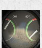
Double gauge: Cylinder Head Temperature and Exhaust Gas Temperature.
