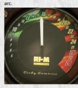
Propeller RPM indicator.
