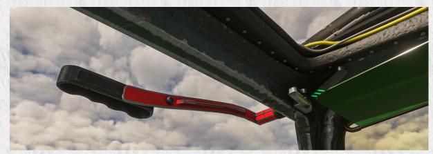
On this picture, you have the flaps retracted (red lever up) and the automatic flaps retractor is already armed.
