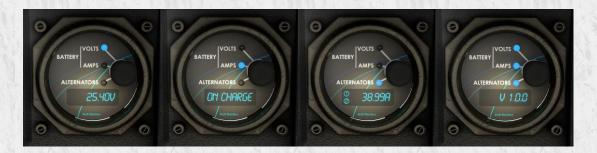
If you take too long to start the engine, or if the alternators are off, or even if the engine is not running fast enough, the battery will discharge, and systems will be shutting down one after the other. Each circuit has its own minimum required voltage.
