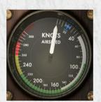
Airspeed – in knots. Taxi in the blue arc and flaps/gears extended not above the white
